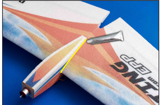
0.10 Glue together the wing and fuselage together, and put the servo wire inside the cabin.
