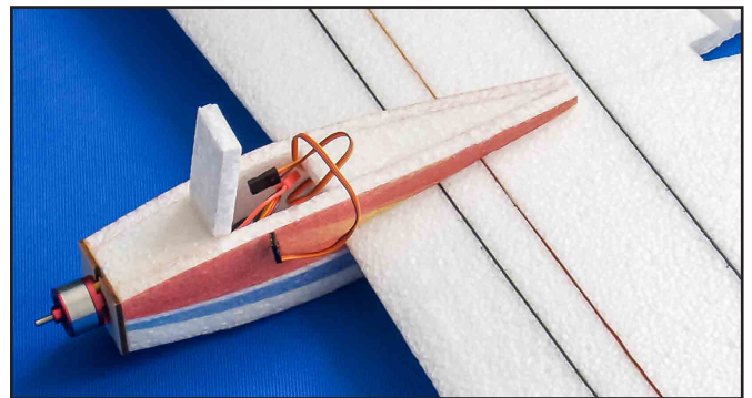
0.11 Paste and glue the vertical tail, keep on the same line with fuselage.
