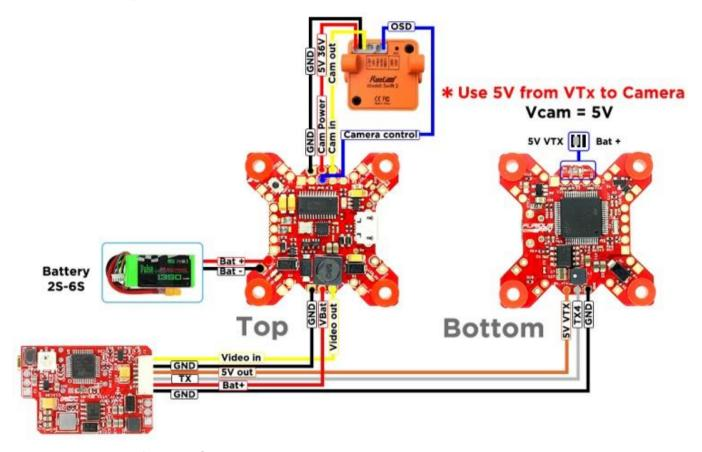
Using battery from VTx to power camera
