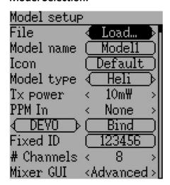
To enter the model setup, press the ENTER button and select Model Menu > Model setup. From here you can create or load models. Model name can be input and the default icon also selected. Model type can be selected to suit your model. TX Power can be adjusted. 10mw-30mw is suitable for most small models. Below the "PPM In" you will find the protocol selection function. Here you can choose one of the many protocols available. The Bind button is used to start the binding process.
